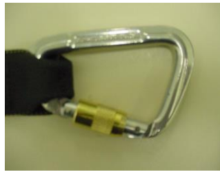
Photo 8: Karabiner gate unsecured. Barrel lock unscrewed.
