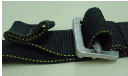
Photo 9: Adjuster hardware showing correct webbing routing.
