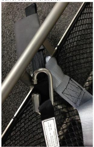
Tighten barrel finger tight then ¼ to ½ turn with tool.
