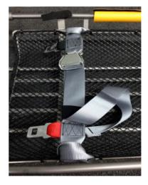
Insert Maillon Delta Ring onto PRS-1A, PRS-1F, PRS-4A & PRS-4F. Ensure ring captures both webbing & barrel closes towards the base of stretcher to avoid loosening from vibrations.
