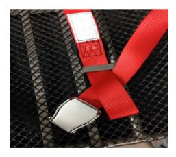
Pull tight ensuring webbing & fastener tab is through loop. Connect to PRS-3 diagonally across stretcher.
