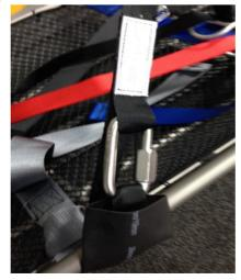
If using a heat shrink or other types of cover over the maillon rapide links, ensure the cover allows a visible inspection of the webbing end loops. Locate the cover centrally over rapide link & shrink down with heat gun. The heat shrink cover reduces damage potential & keeps correct orientation of the maillon rapide by preventing side loading caused when the maillons rotate through the webbing loops. It also assists in preventing any loosening of the barrel.
