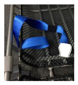
• Route the hardware end through the loop towards the middle of the stretcher.
