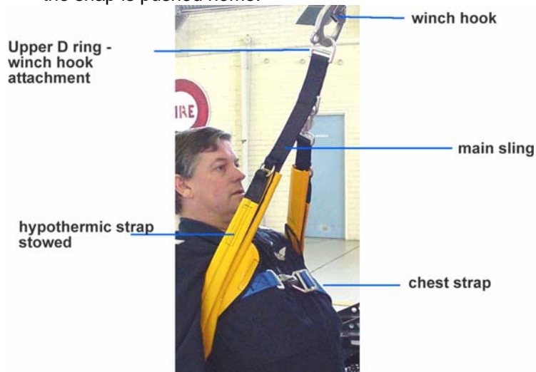
Diagram 1: Fitting the Rescue Strop
