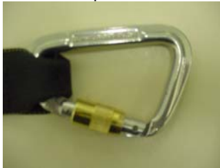
Photo 8: Karabiner gate unsecured. Barrel lock unscrewed.
