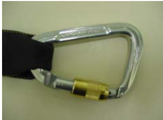
Photo 7: Karabiner gate secured. Barrel lock screwed up.
