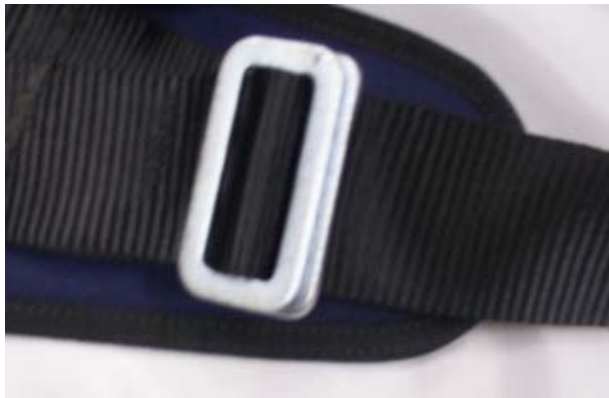
Diagram 13: HW-CRW [-3] leg strap hardware coupled correctly.
